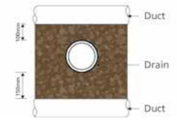
Minimum clearance between duct and drain
